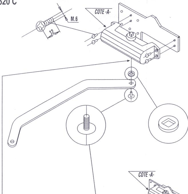
NB. L'ASSEMBLAGE DE CES DEUX PARTIES PEUT SEMBLER DIFFICILE A CAUSE DES MULTIPLES COUCHES DE PROTECTION. PRESENTER LA BRAS DE LEVIER SUR L'AXE ET EFFECTUER LA JONCTION AVEC LA VIS.
